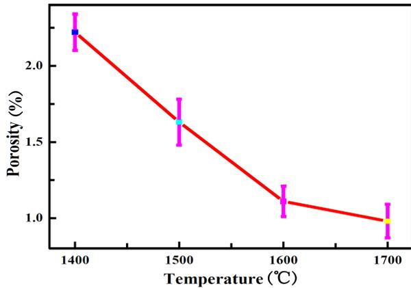
Figure 3. Porosity of PcBN samples at different sintering temperatures
