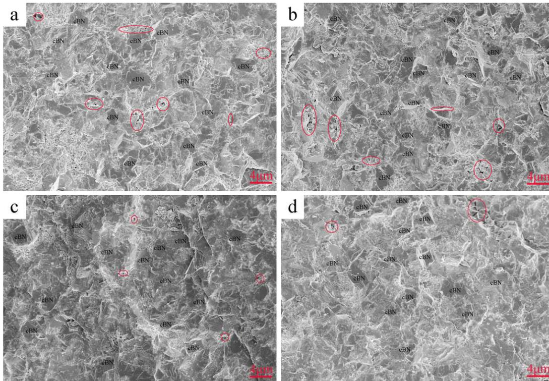
Figure 2. SEM of the PcBN samples sintered at different temperatures: a) 1400 °C, b) 1500 °C, c) 1600 °C and d) 1700 °C
