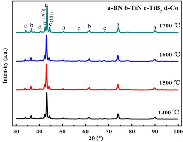
Figure 1. XRD of the PcBN samples at different sintering temperatures
