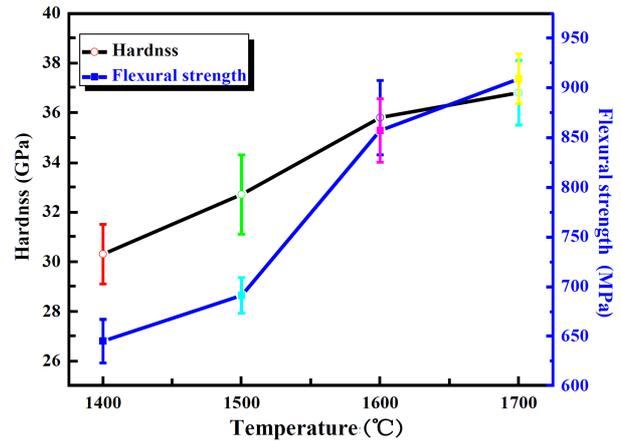
Figure 4. Mechanical properties of PcBN samples at different sintering temperatures
